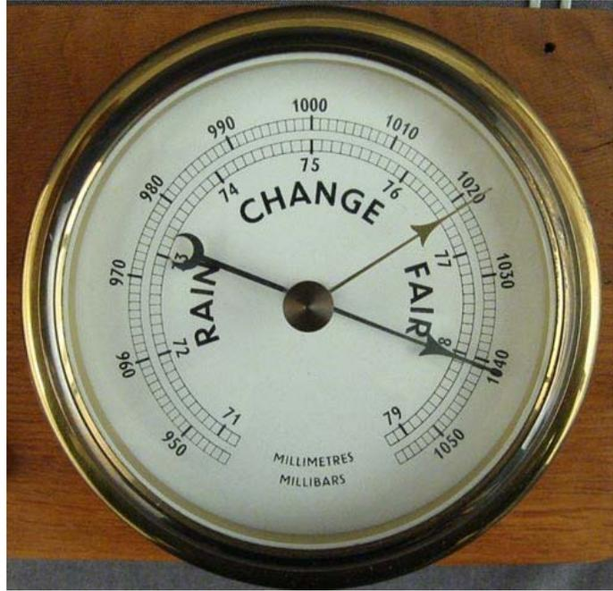
**Figure 6: A Barometer - for measuring atmospheric pressure (Source: Langspeed)**
